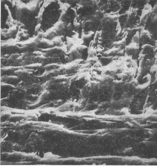
PLATE 1 Surface of radial section wood.
